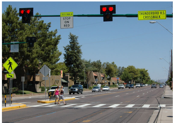
HAWK signal with pedestrian refuge, striping, and signage
